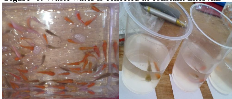
Figure-7: Toxicity of thus collected water is tested by measuring survival time of fish
